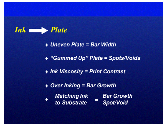
Fig. 8: Flexographic printing process errors
