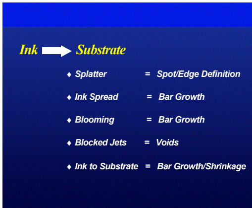
Fig. 7: Ion Deposition printing process errors
